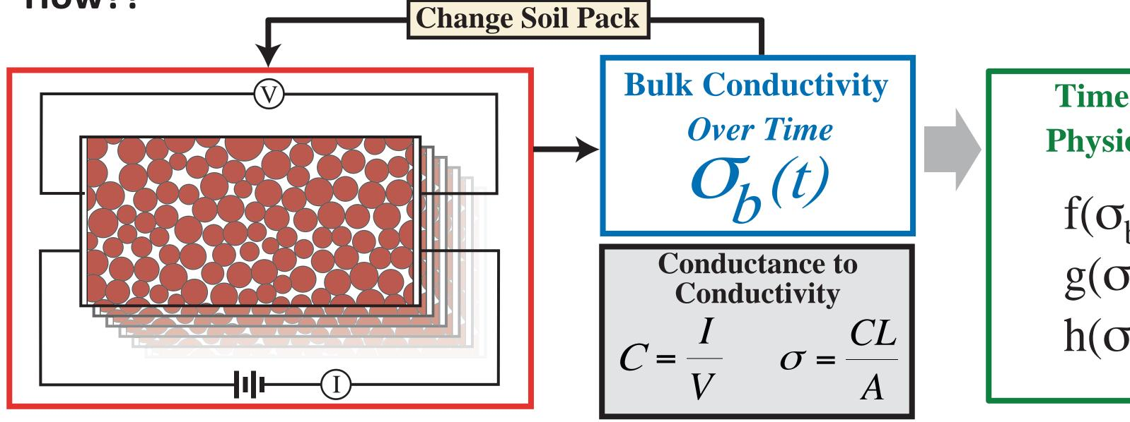
**Treat the earth as a simple circuit** and use the conductance (*C*) to calculate the conductivity ( $\sigma_{\rm h}$ ). Use **rock physics** to relate conductivity to a parameter of interest.
